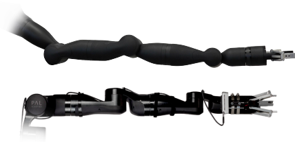
Fig. 3. New TIAGo arms with Series Elastic Actuators
