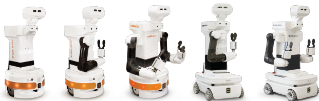
Fig. 1. Different configurations of the TIAGo robot. Left to right: TIAGo Lite, TIAGo, TIAGo++, TIAGo OMNI and TIAGo++ OMNI
